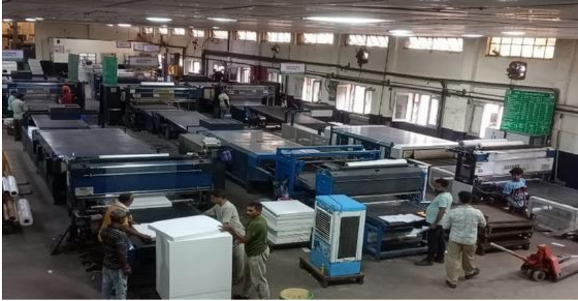
Infeed Conveyors of Ream Packing
